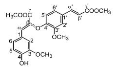
An  $\alpha = \beta$ -*O*-4'-enol ether dimer of methyl ferulate obtained from outer bark of *Quercus variabilis*
