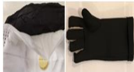
Facemask and Glove filtering applications of CNT hybrid material
