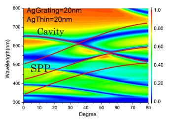
Simulation results of the PTS device showing two possible Exceptional Points (EP) at @30° and 54° when both the Ag grating step is 20nm deep and Ag thin film is 20 nm thick.
