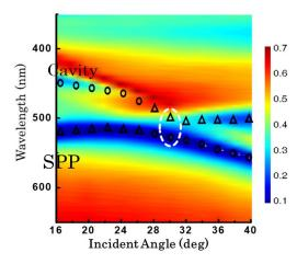
Microcavity-SPP mode coupling with Rabi-like split. The microcavity has a passive dielectric.
